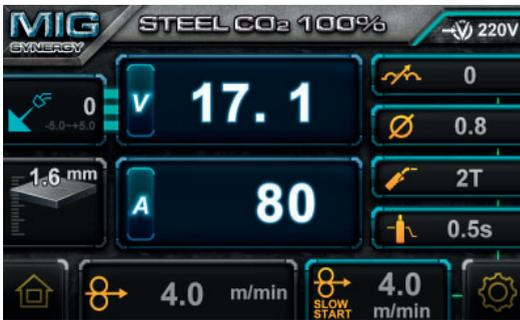
To adjust the voltage independently, Rotate Left Knob (1) to adjust the welding voltage. This will change and give the display screen as below.
