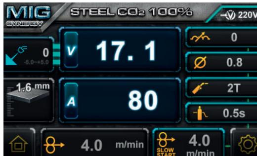
Then use the Left knob (1) to adjust the welding voltage -5~+5V from the standard synergic setting. This will not change the wire speed. It is recommended for ease of use that the wirefeed target speed is adjusted first and then the voltage setting fine-tuned if necessary. Refer to the Welding Settings Quick Reference Chart on page 21 and inside the wirefeed door for recommended common settings.
