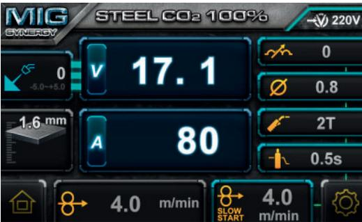
2T/4T function: press the Right Button (4) ,2T/4T Selection Switch to move between 2T and 4T modes. 4T operation means the trigger is pulled once to start welding and pulled again to stop. This is useful for long weld joints. 2T mode, the trigger must be depressed and held during welding.
